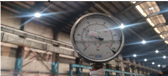
Hydrostatic test control
