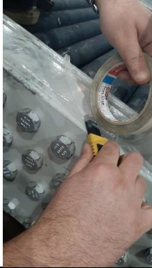
Paint adhesion test control
