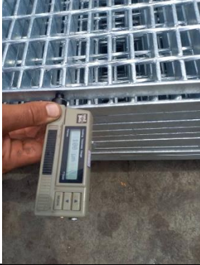
Coating thickness control
