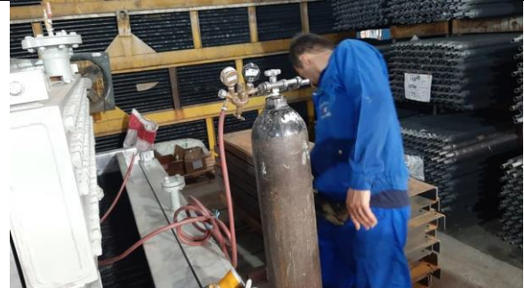
N2 Purging control
