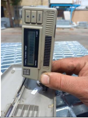
Coating thickness control
