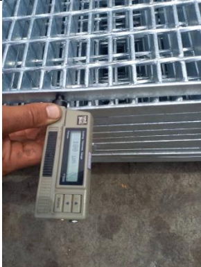
Coating thickness control
