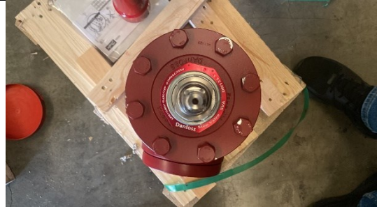
Inspection of 2nd Compressor - Spares (Head of Bolts needs touch-up before shipment)
