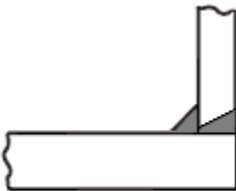
Abutting/Set-on Nozzle No Pad
