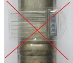
Figure 3: Not correct IQI placement
