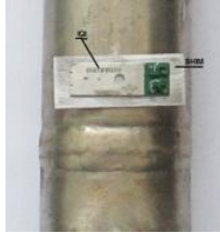
Figure 1: Hole type IQI
