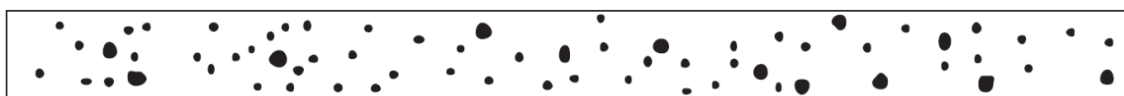
(a) Random Rounded Indications Typical concentration and size permitted in any 150 mm length of weld.
