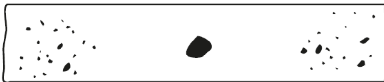
(a) Random Rounded Indications Typical concentration and size permitted in any 150 mm length of weld.
